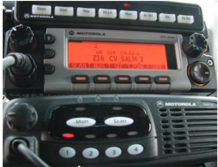
Shown are a STARS [XTL 5000](#) and a [CDM750](#) SIRS radio installed in a VSP vehicle at a division open house in Salem. STARS installations also include the siren/light controller (at top). The XTL 5000's display shows:
